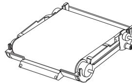
Make sure to set the ink ribbon roller to the ditches firmly.
