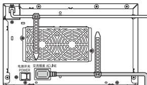
Securing hole for the cable tie
