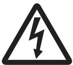
The lightning flash with arrowhead symbol, within an equilateral triangle, is intended to alert the user to the presence of uninsulated “dangerous voltage” within the product’s enclosure that may be of sufficient magnitude to constitute the risk of electric shock.
