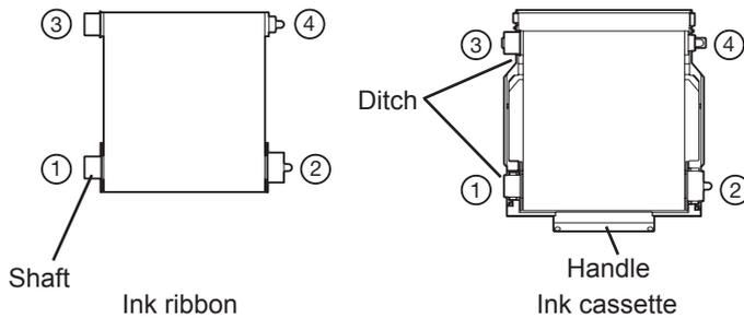
Make sure to set the ink ribbon roller to the ditches firmly.
