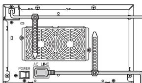
Securing hole for the cable tie
